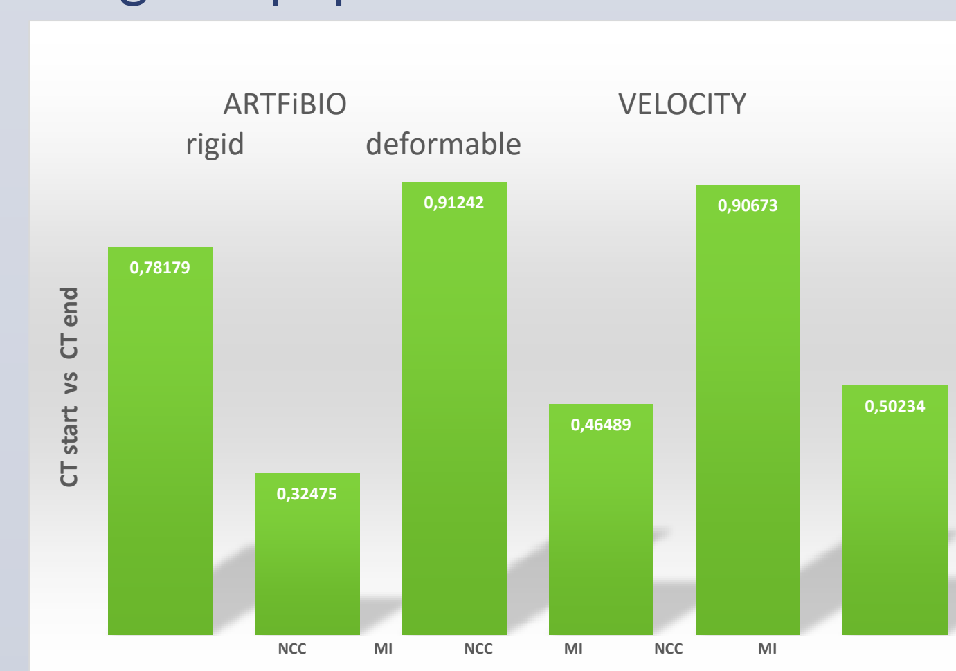
Fig.3 In this figure we compare the register between 2 X-ray CT made whit our home software (ARTIFIBIO) versus commercial software Velocity®. For this we use NCC and Mutual Information metrics
